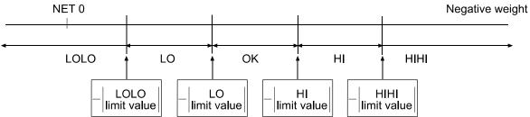
Note: To start the take-away check weighing, be sure to use the TARE key to tare the weight of the container filled with objects. The ZERO key may zero the display, and the scale goes below the zero point by taking out the objects. Then, the auto-tare function or TARE key does not work.
