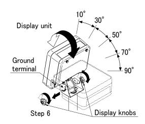
The display unit can be adjusted in five steps in the up-and-down direction. Setting the display sideways is also possible. (Make sure that the pole is secured at the lower part of the pole using the hex screws. Do not turn the display unit at a joint for the pole.)
