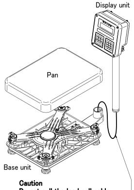
Do not pull the load cell cable.
