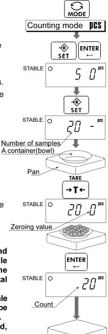
Note The pan shape depends on the scale model.
