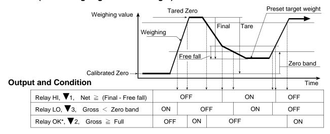
\* Relay OK output can be changed to OVER or UNDER by setting F24. Triangle 2 is displayed when Gross ≥ Full regardless of the F24 setting. OVER/UNDER is judged always and the result is output to the display and the relay.
