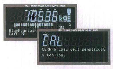
The main display has 18mm tall characters and a 7-digit VFD for the weight value displays.
